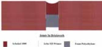
Recommended for use in expansion joints in brickwork and blockwork.
